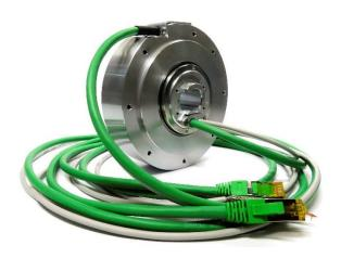
The contactless data transmission channel offers improved lifetime and reliability without the need for maintenance. The contactless design guarantees error free data transmission even at very high rotating speeds. The IRT version supports PROFINET class C and other real time protocols. The data transmission channel is realized by a rotating capacitive coupler.
