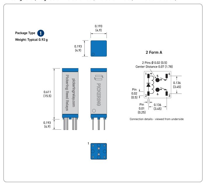
**Important:** Where the optional internal diode is fitted, the correct coil polarity must be observed, as shown by the + symbol on the schematic.
