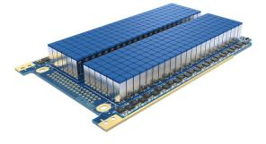
A total of 288 Series 125 relays on a Pickering Interfaces PXI BRIC daughter card illustrates the packing density of these extremely small Reed Relays.
